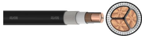
POLYCAB BS 6724 MC SWA LSZH - Power Cable, 0.6/1 KV AC
